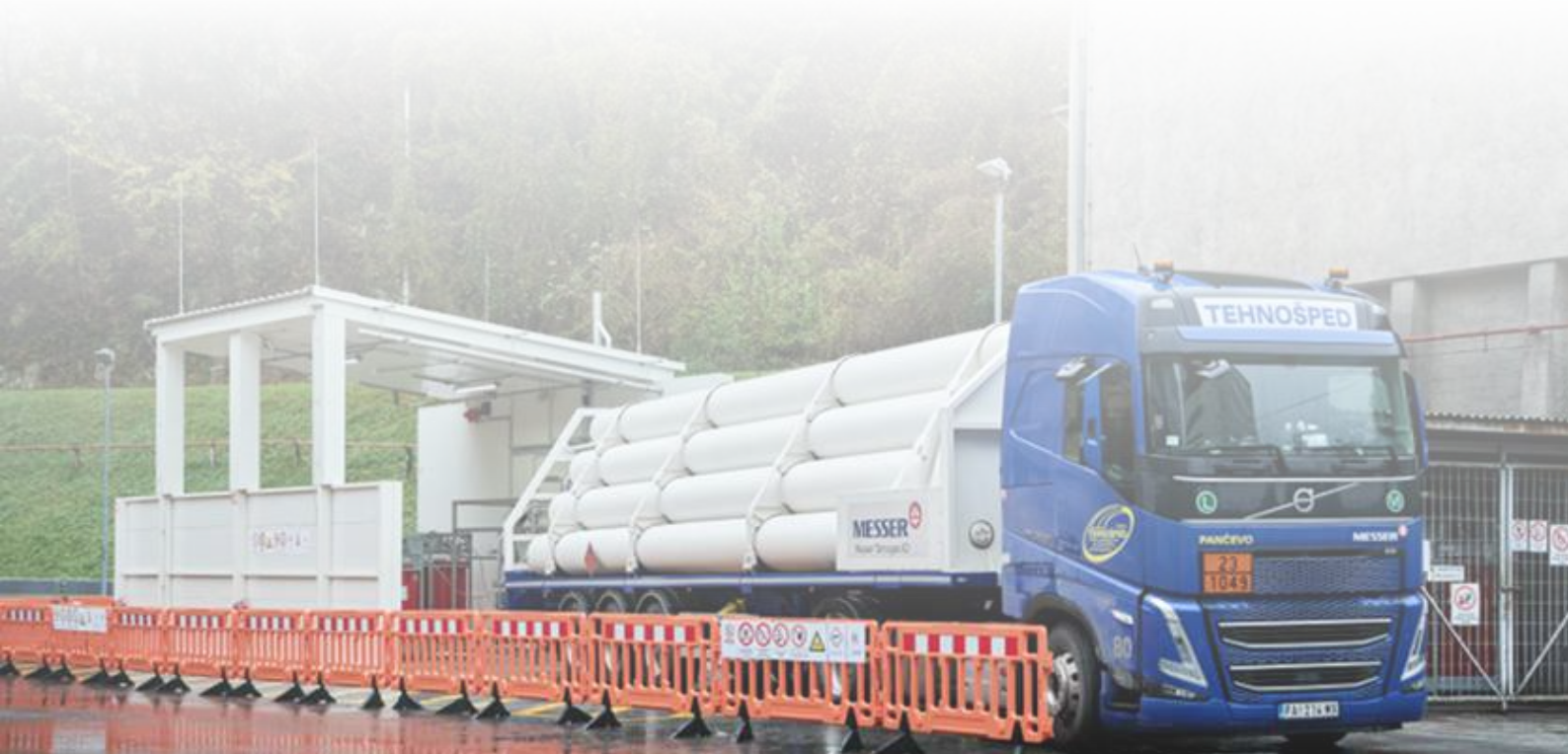
Figure: Supply of hydrogen for the glass furnace
